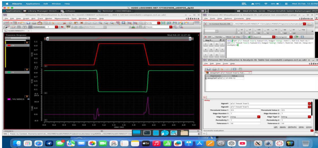
Fig. 2. Measured transient waveform for FO1 showing t_{PLH} = 21.05 ps.
