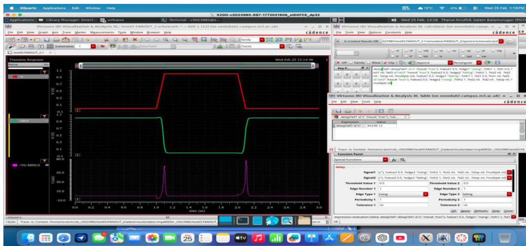
Fig. 4. Measured transient waveform for FO2 showing t_{PLH} = 34.63 ps.
